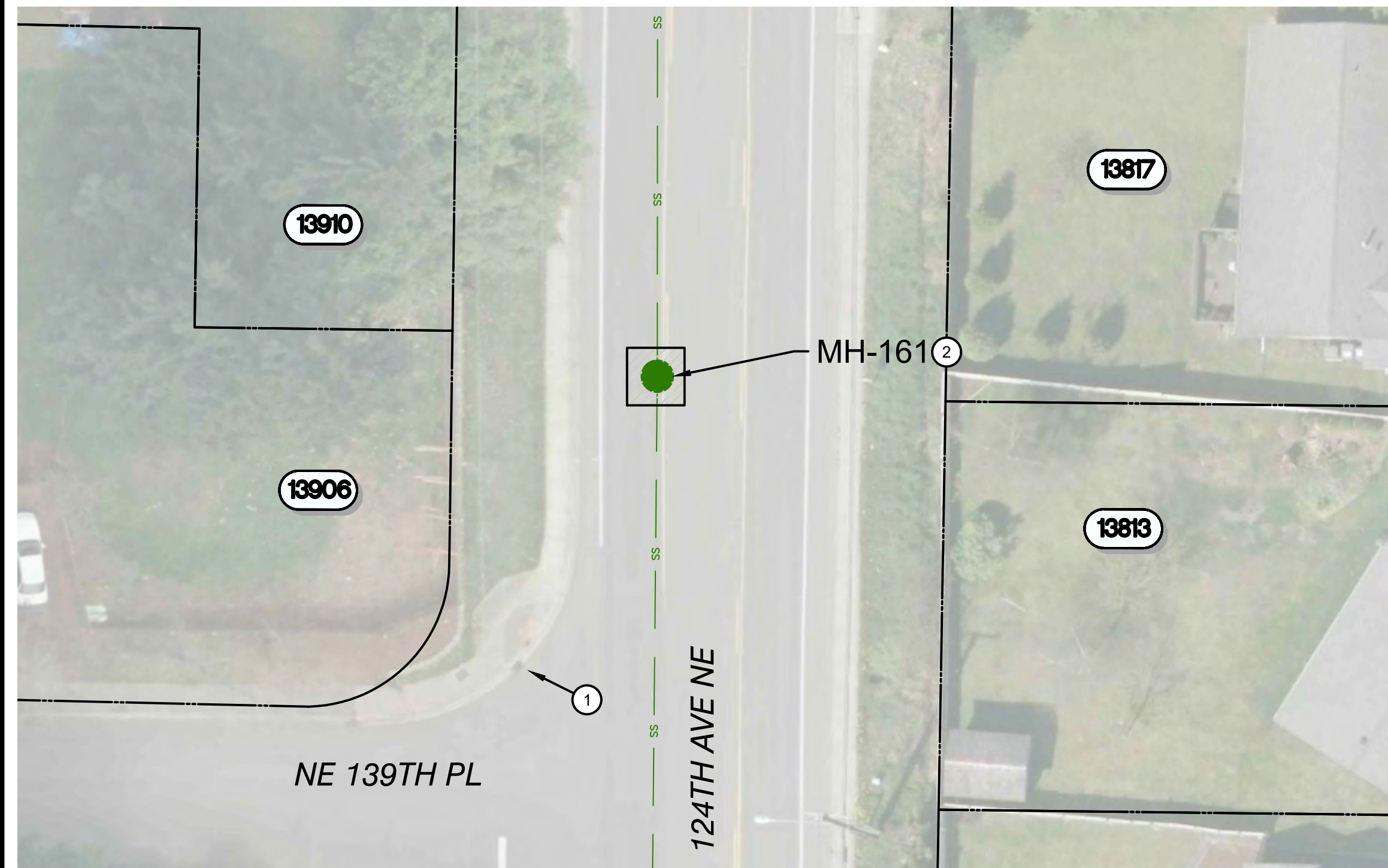
MH - 161 - REPLACE FRAME, COVER AND 18" OF ADJUSTMENT RINGS.
