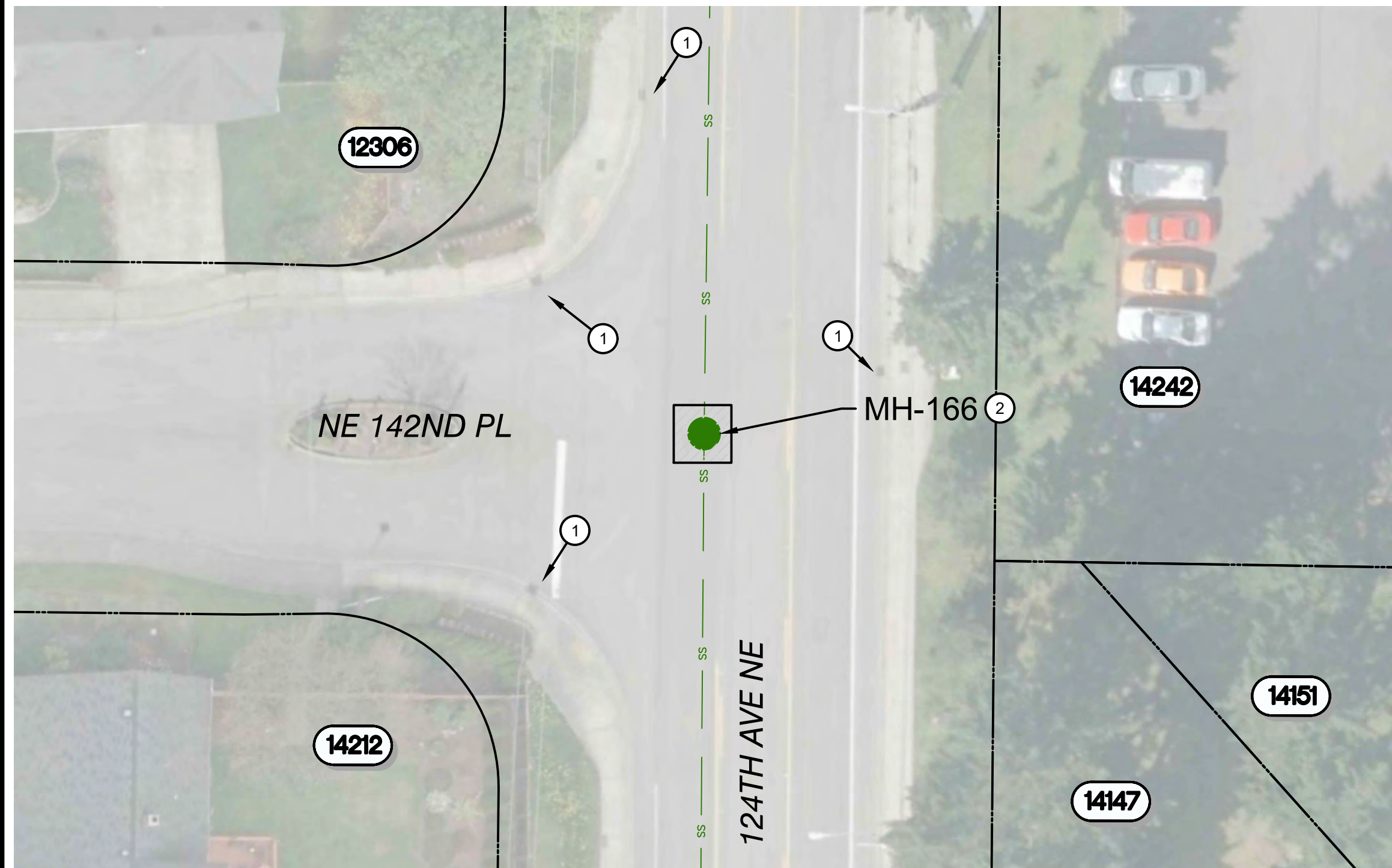
MH - 166 - REPLACE FRAME, COVER AND 8" OF ADJUSTMENT RINGS.
