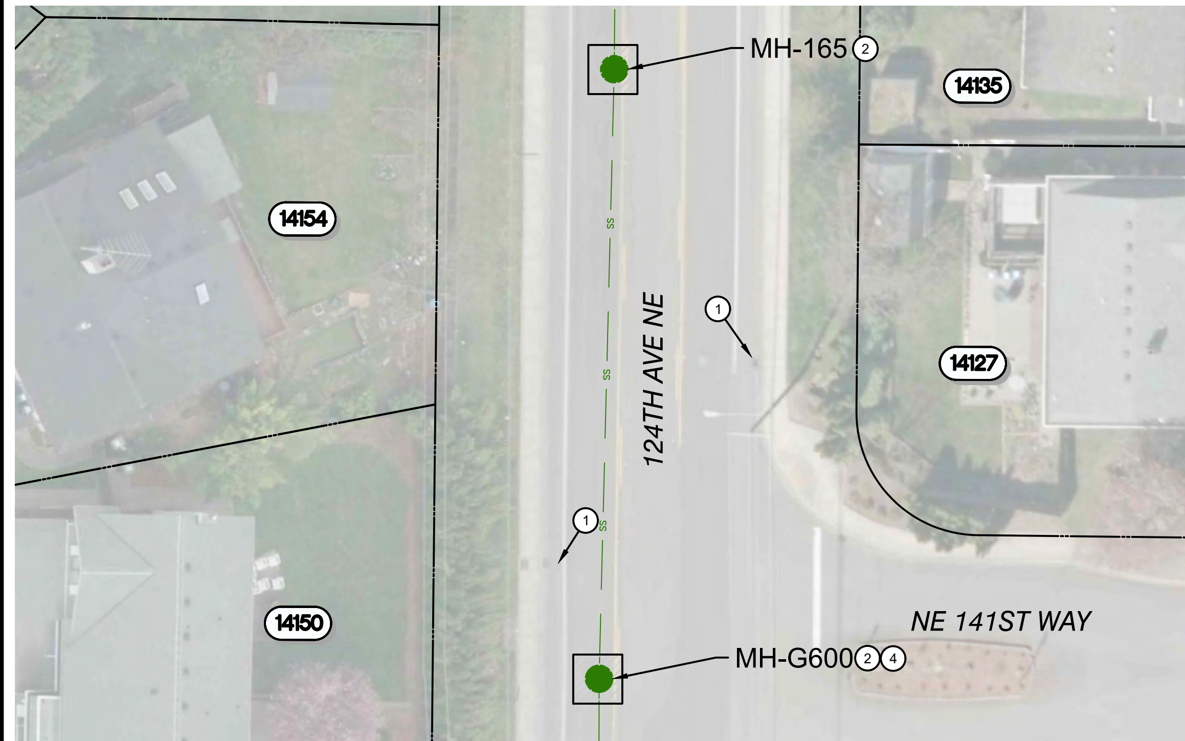
MH - 165 - REPLACE FRAME, COVER AND 10" OF ADJUSTMENT RINGS.
