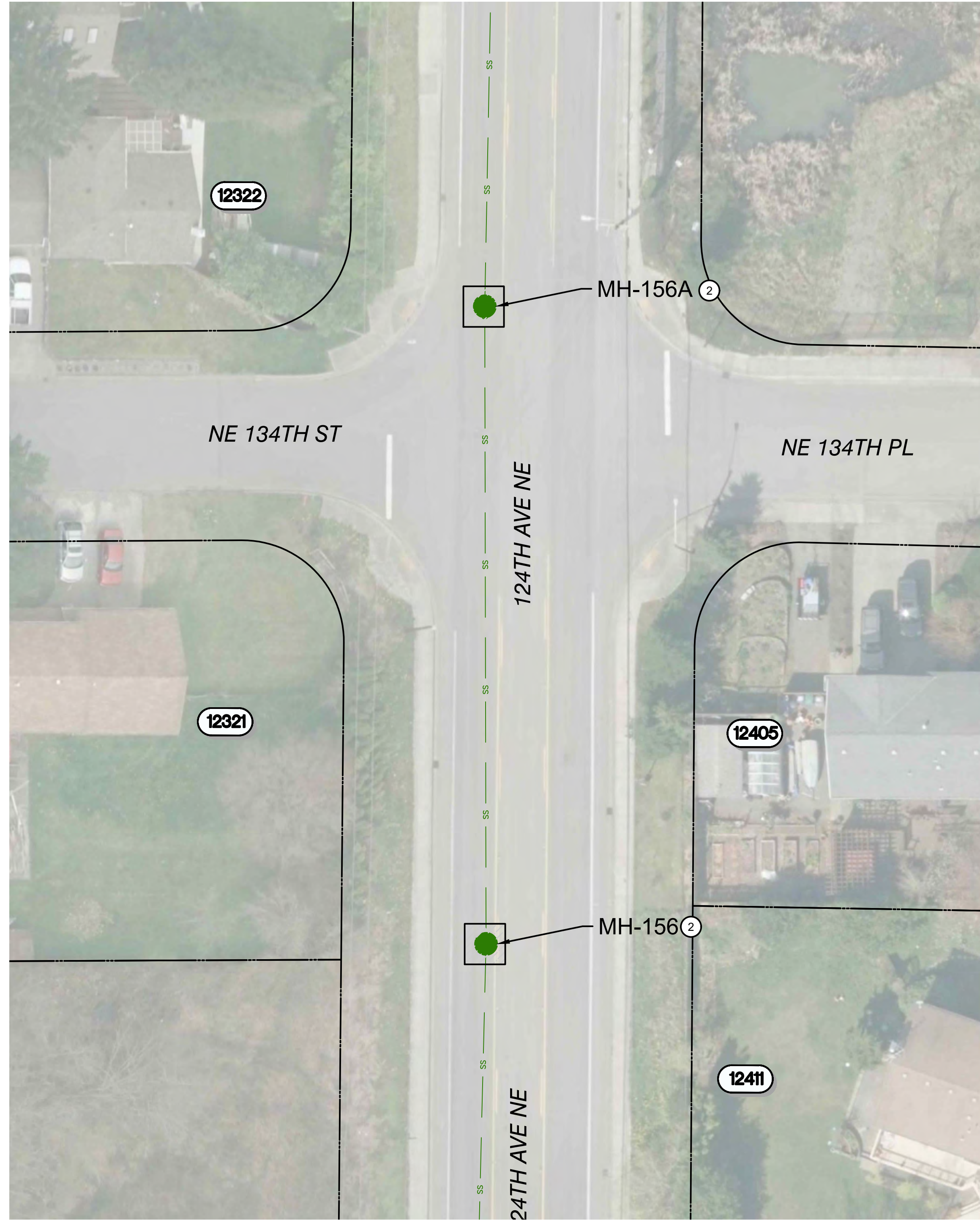
MH - 156A - REPLACE FRAME, COVER AND 10" OF ADJUSTMENT RINGS.
