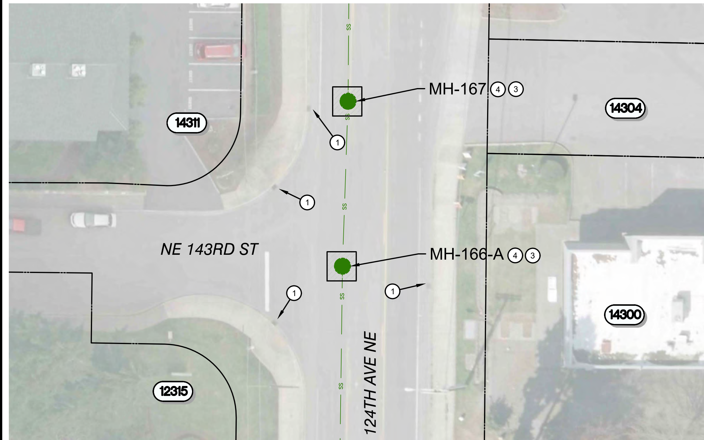
MH - 166A - ADD MAHOLE SECTION, REPLACE MANHOLE CONE, FRAME, COVER AND ADJUSTMENT RINGS AS PER DETAIL 3 SHEET 17. CONFIRM KEY-WAY PRIOR TO INSTALLATION. PROTECT SURVEY MONUMENT
