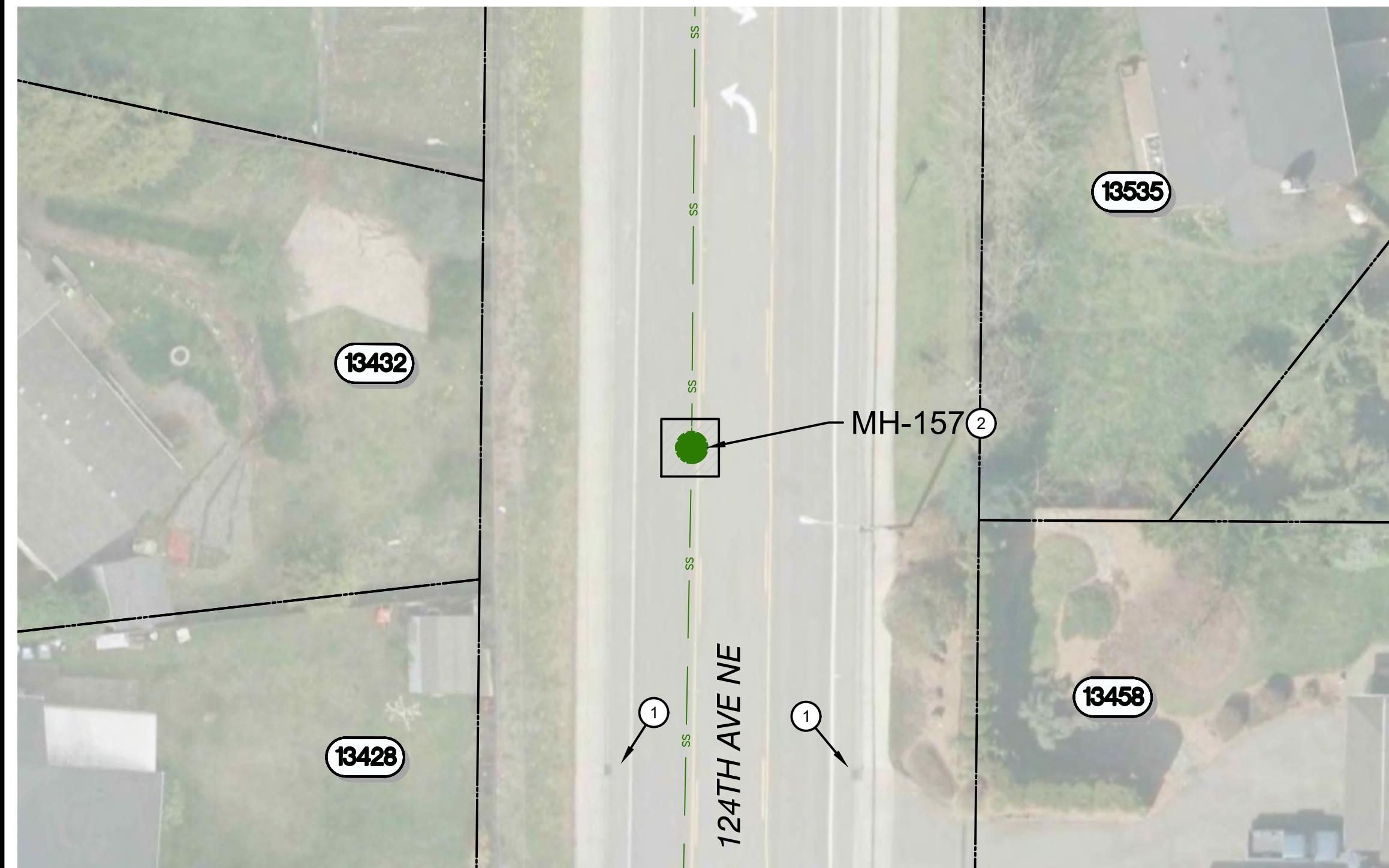
MH - 157 - REPLACE FRAME, COVER AND 8" OF ADJUSTMENT RINGS.
