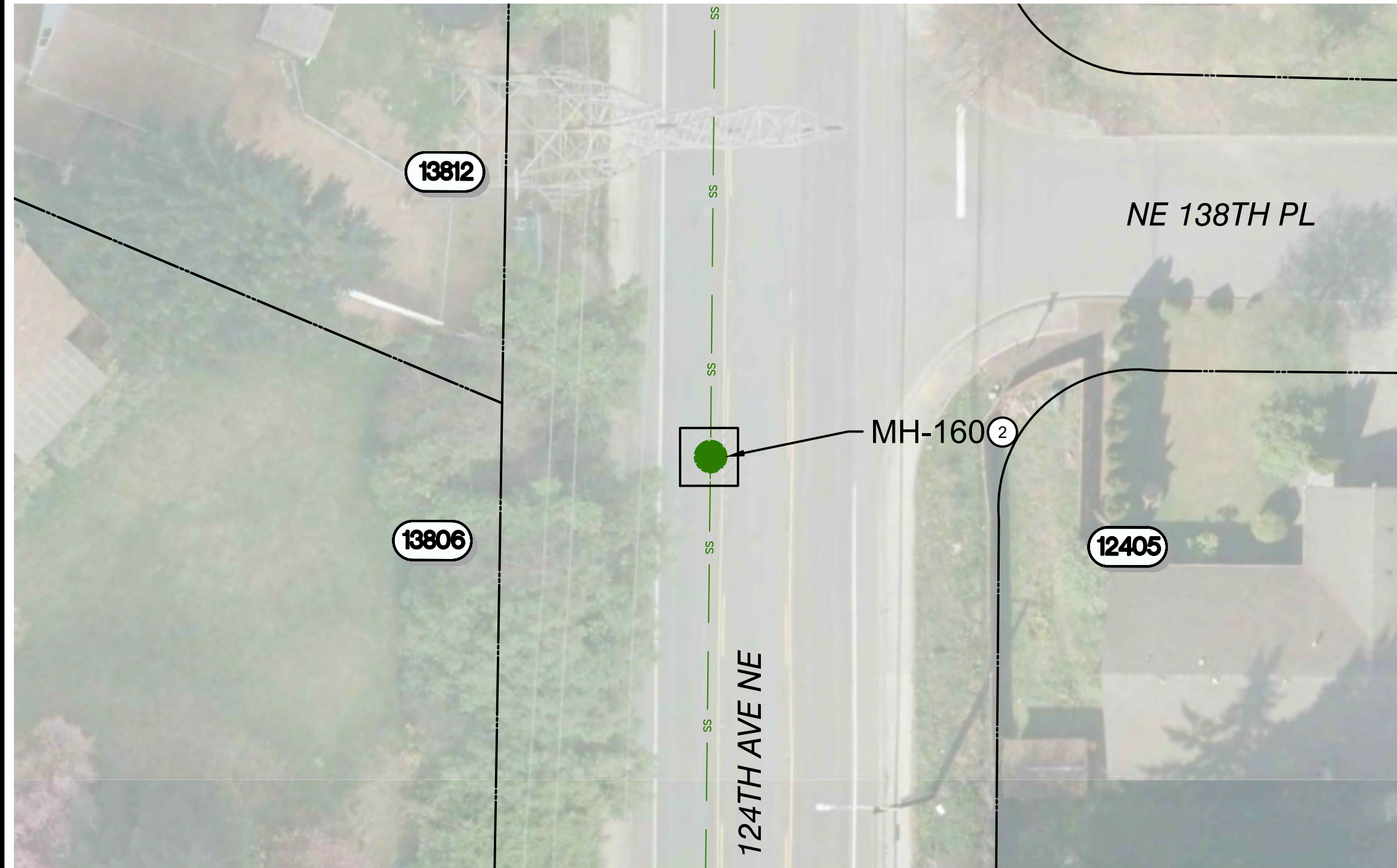
MH - 160 - REPLACE FRAME, COVER AND 18" OF ADJUSTMENT RINGS.
